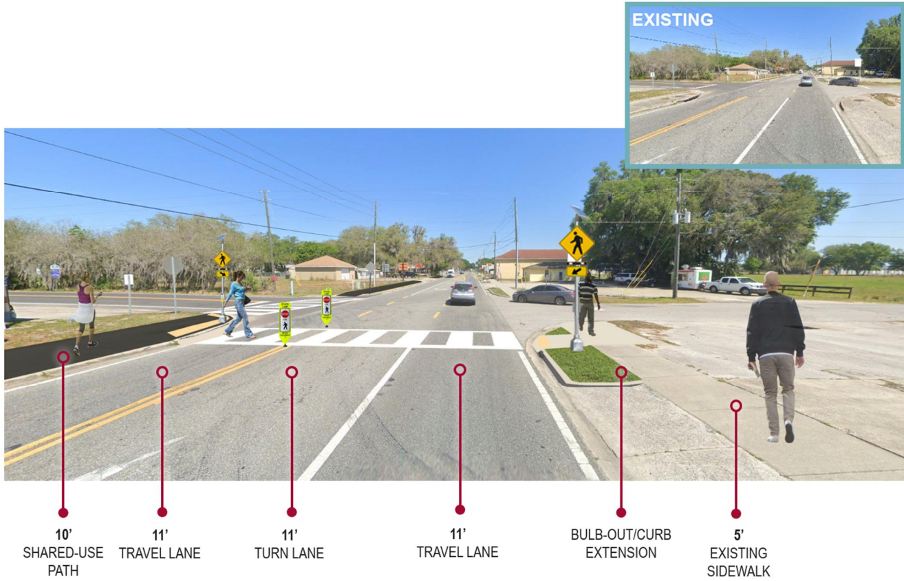
Figure 4-10: Option 1 Cross Section— At C 478/NW 4 th Avenue
