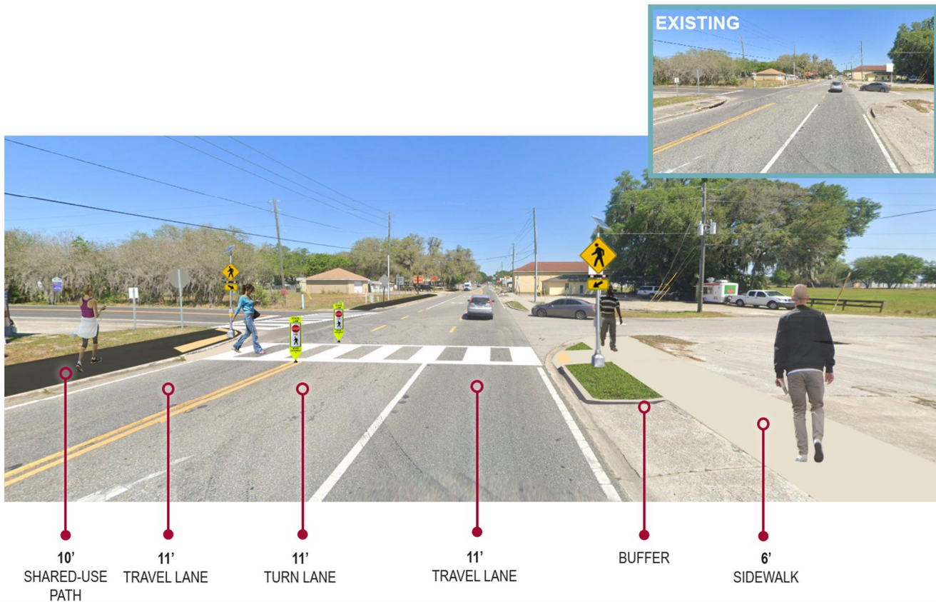
Figure 4-11: Option 2 Cross Section— At C 478/NW 4 th Avenue
