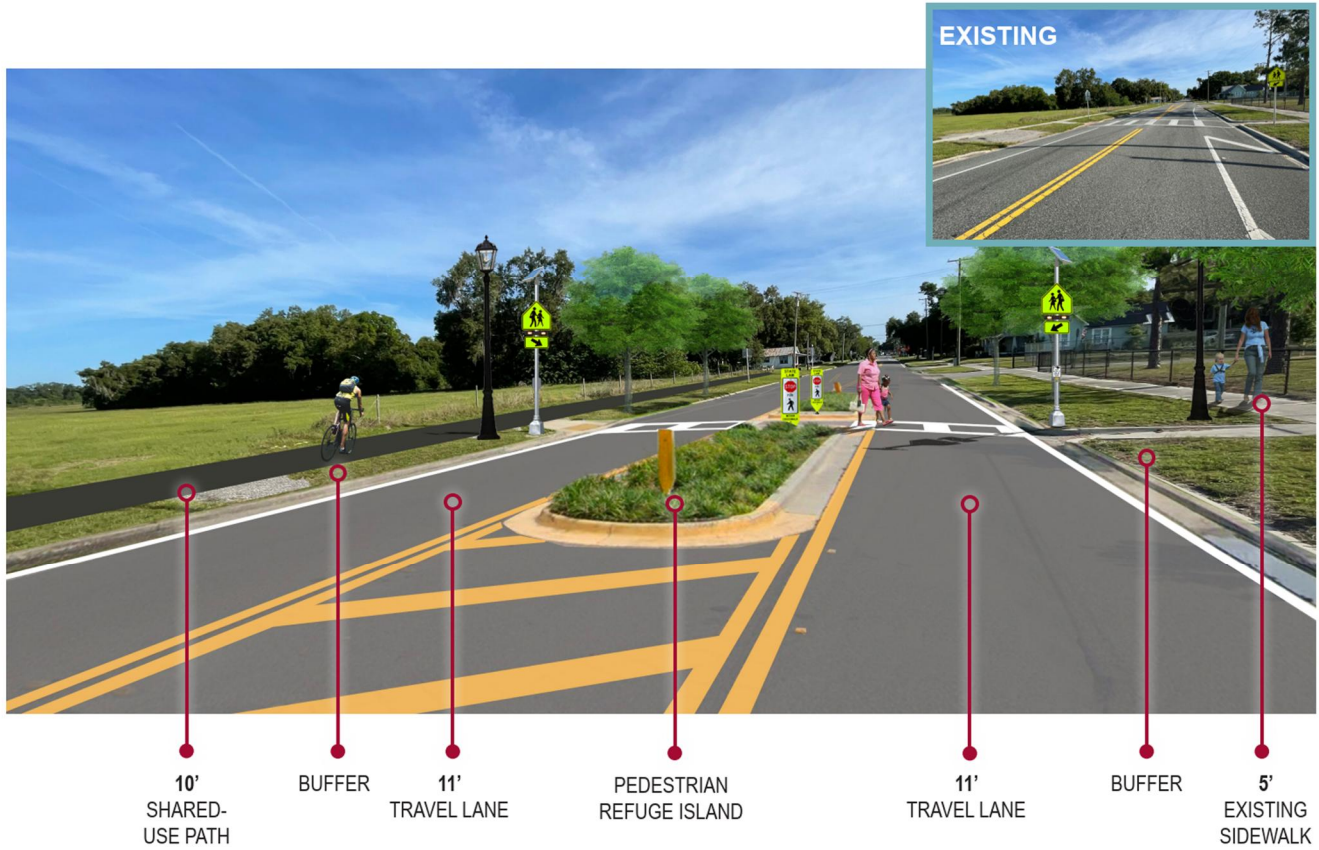
Figure 4-6: Option 1 Cross Section— At Webster Elementary School
