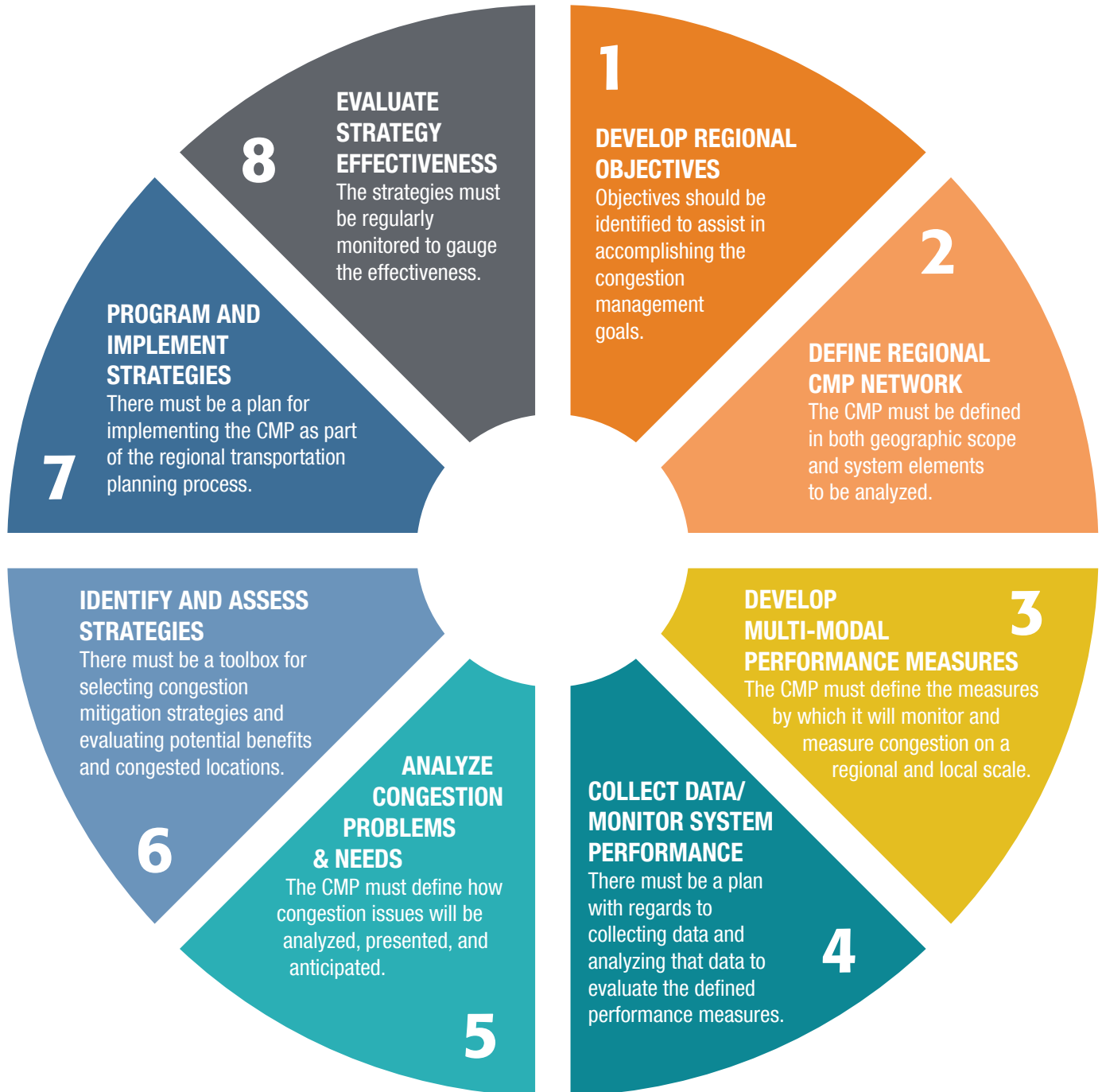
Figure 2. Federal Eight-Step Congestion Management Process
